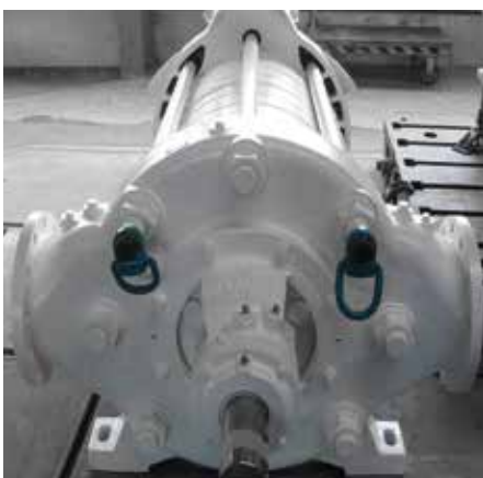
Two flanges in one suction casing
