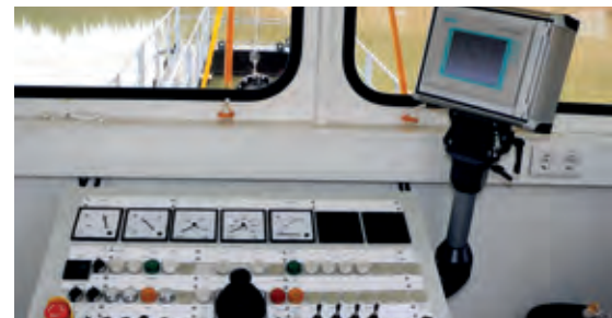
Retrofitting a new PLC suction pipe automation system
