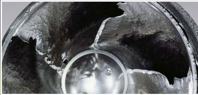
Impeller made of Duplex Stainless Steel
