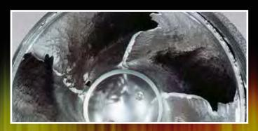
Impeller made of Duplex Stainless Steel
